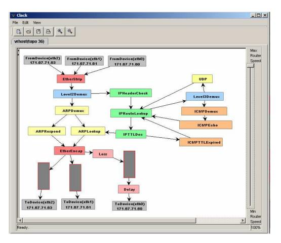
A simple configuration for a router with three interfaces. Packets enter at FromDevice components at the top and exit the router at ToDevice components near the bottom. Components processing at layers higher in the standard OSI model are positioned further to the right and components are logically grouped by color.
